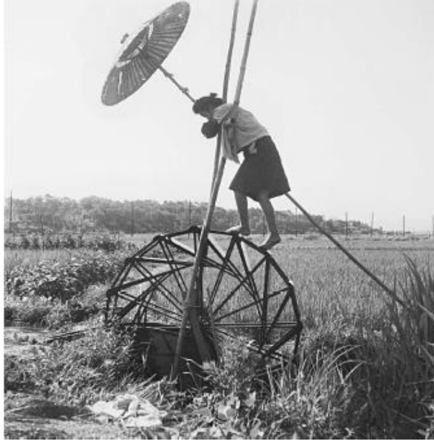
Human-feet powered devices traditionally were used to move water short distances and up low grades. This irrigation wheel in Japan was still being used in 1958 to irrigate a small plot.
